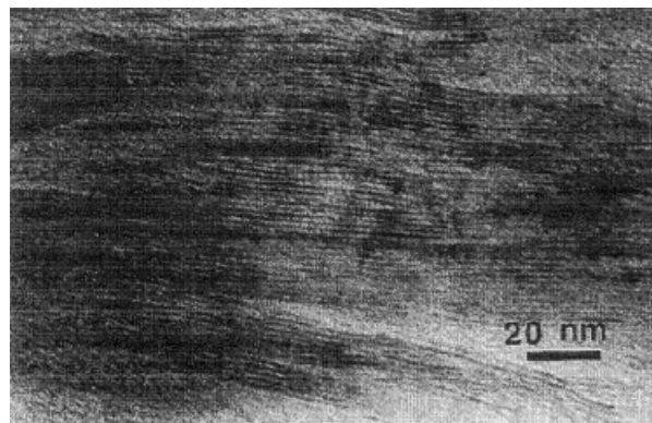
Figure 6 The TEM image of a carbon residue obtained by combustion of a nylon 6.6 nanocomposite. 38
